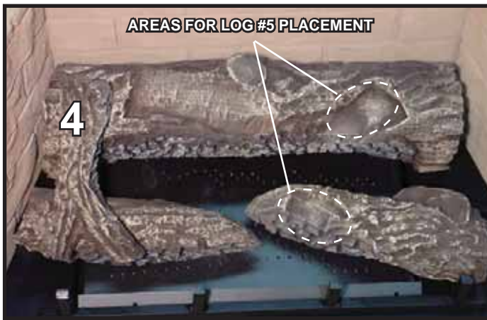
LOG #4 (SRV340-704): Place log #4 across log #1 and log #2 in the grooved out areas as shown.
